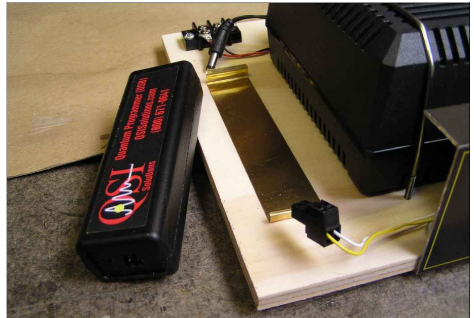
Photo 2 — The Quantum Programmer is held in place by a brass spring clip to permit easy removal for other applications.
