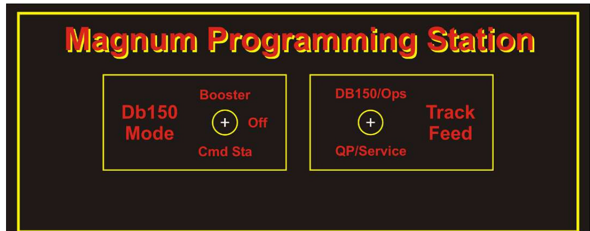
Figure 1 — The author's front panel layout, shown full size (2.5 "x 6 "). The original was created in CorelDraw, then printed on white inkjet decal paper from BEL , Inc., and overlaid with several coats of Krylon aerosol crystal clear satin finish.
