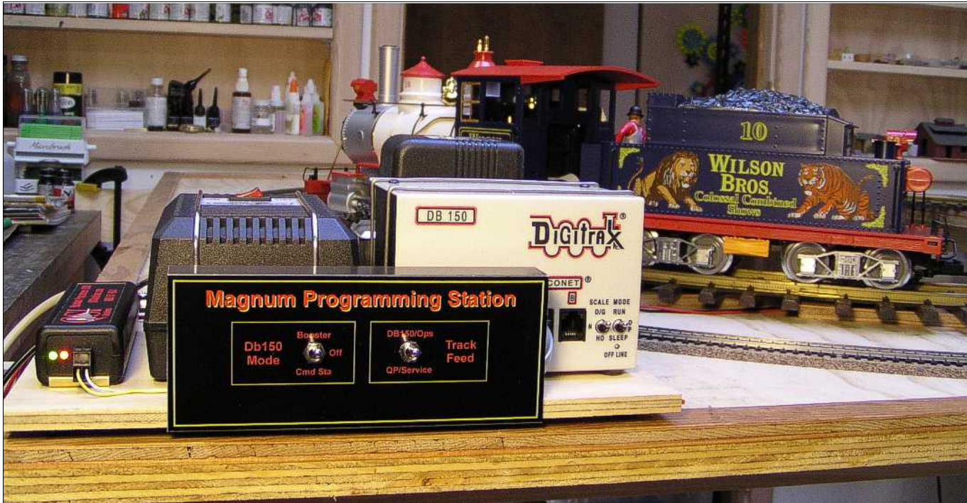
Photo 3 — The Magnum Programming Station in use testing and programming a QSI Solutions Magnum decoder installed in an older LGB Mogul steam locomotive.
